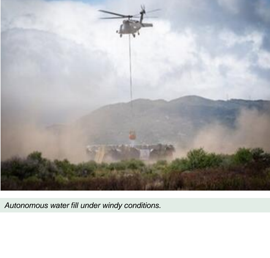
Autonomous water fill under windy conditions.
