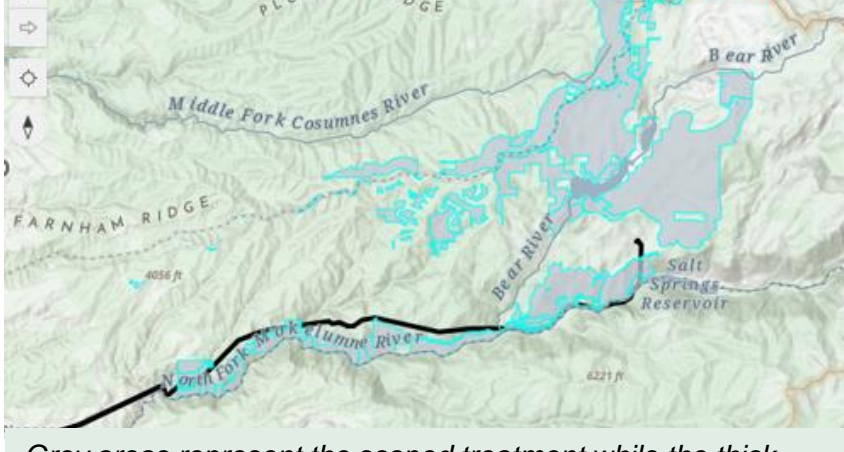
Grey areas represent the scoped treatment while the thick black line represents PG&E transmission and generation assets. The dotted line is an important access road.
